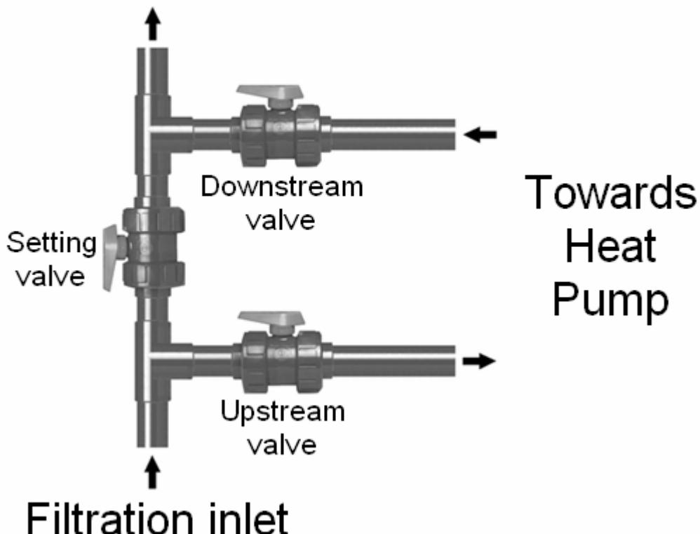
Warning, the by-pass must be fixed on a wall or on a support, so that by-pass and tubes weight is not supported by the heat pump connexions!
