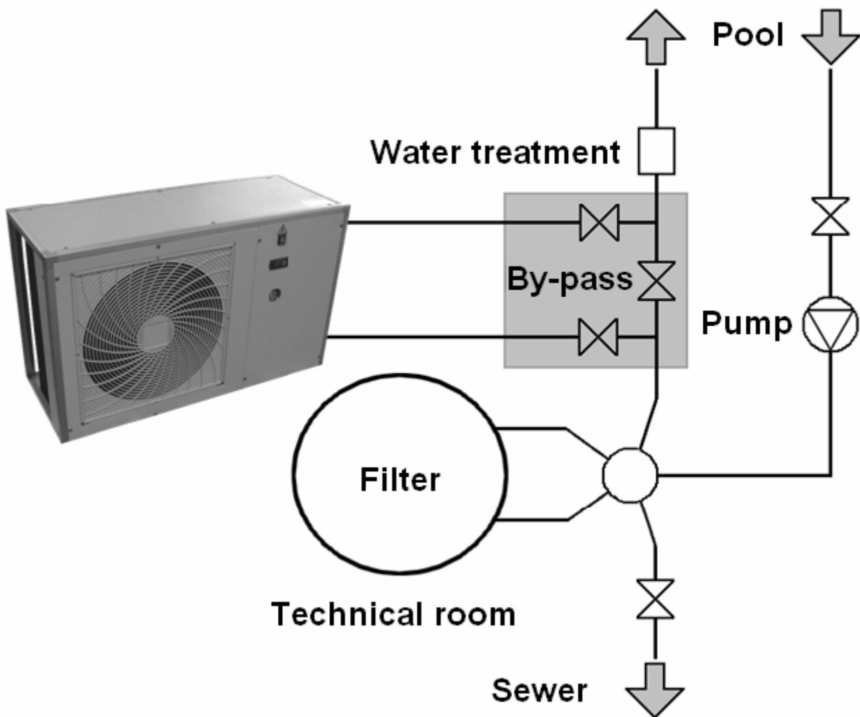
If your installation is equipped of a water treatment with product adductions (chlorine, brominates, salt...) the by-pass must be installed before the water treatment, with a non-return valve between the by-pass and water treatment.
