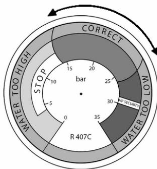
To optimize the performance of heating and energy saving, it is advisable to regulate the water flow through the pool heat pump.
